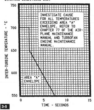
All conditions except starting: if the inter-turbine temperature (ITT) exceeds 700°C during takeoff, or if 680°C is exceeded at any time other than takeoff, refer to Chapter 77 of the Maintenance Manual and Engine Maintenance Manual.
