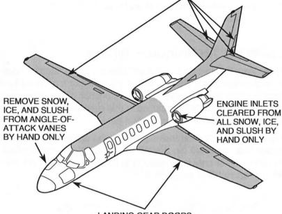
LANDING GEAR DOORS AND WHEEL WELLS MUST BE FREE OF SNOW, ICE, AND SLUSH
