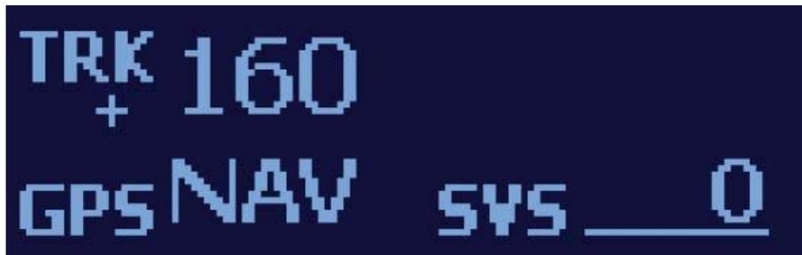
**Vertical Speed** can be adjusted by a momentary press and release of the KNOB to move the cursor under the number next to SVS, and then rotating the KNOB.
